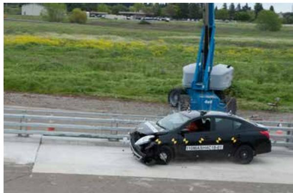
Image 1: A 2,420 pound small car impacting at 62 miles per hour (mph) and 25°
