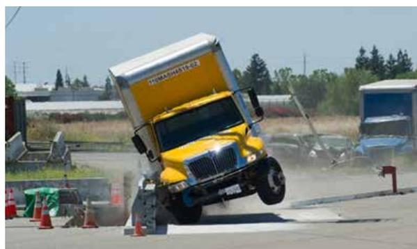
Image 3: A 22,000 pound single-unit truck impacting at 56 mph and a 15°.
