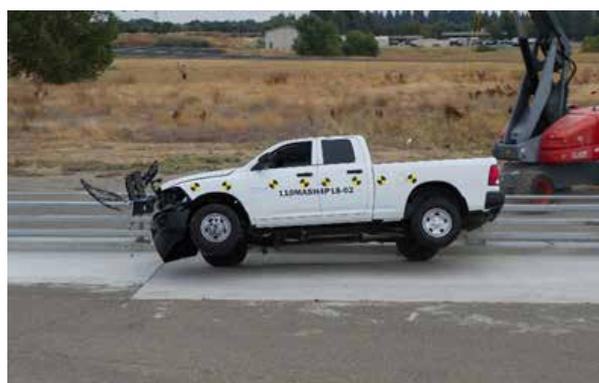
Image 2: A 5,000 pound pickup truck impacting at 62 mph and 25°.
