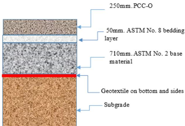
Figure 2: Concrete Test Section Design
