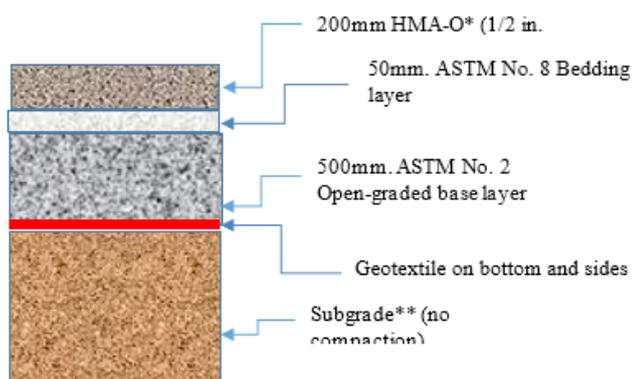
Figure 3: Asphalt Test Section Design
