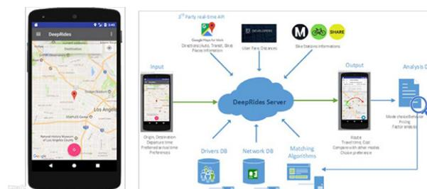
Image 2: Passenger mobile app (left) and its system framework
