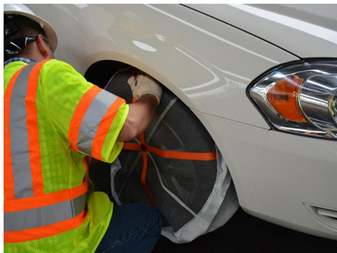
Cloth tire traction control device being installed on the car
