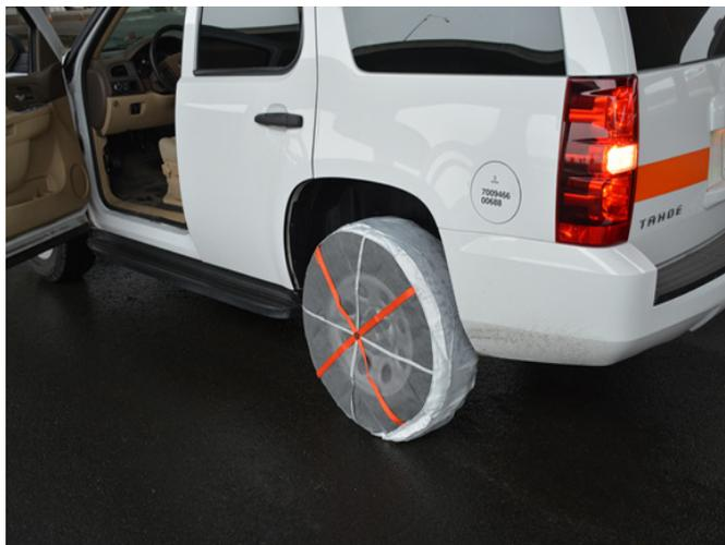
SUV with the cloth tire traction control device installed on the rear wheels
