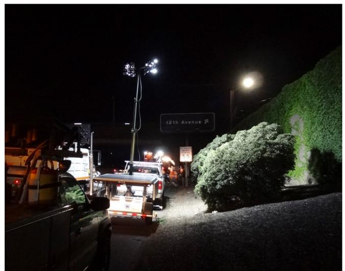
Figure 2: Wanco Solar Light Trailer Caltrans West Sacramento Field Test
