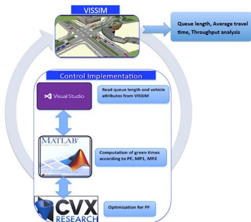
FIGURE 4: Overview of the implementation of control architecture with Verkehr in Städten - Simulations Model (VISSIM)
