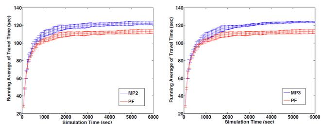
FIGURE 5: Comparison of the running average of travel time for heavy traffic under proportionally fair (PF) and max pressure (MP) controllers
