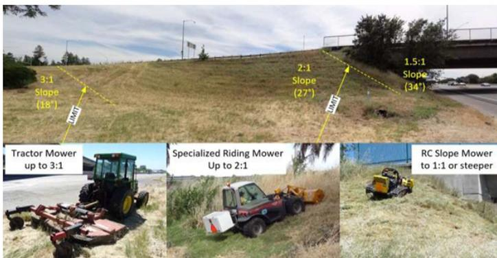
Figure 2: Mowers on typical roadside slopes
