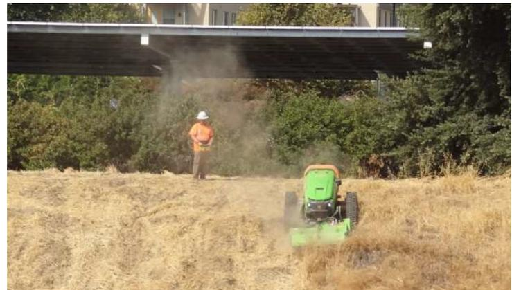
Figure 3: RCM mowing downward from top of 2:1 slope
