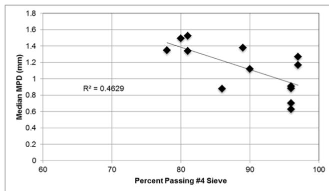
Image 3: Correlations of percent passing the #4 sieve and median MPD (mm).
