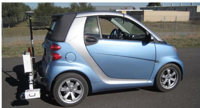
Image 2: Vehicle mounted high speed inertial profilers used for macrotexture and roughness measurements.
