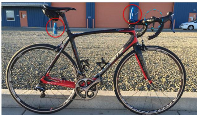
Image 1: Road bicycle instrumented with accelerometers (solid red circles) and a Global Positioning System (GPS) unit on the handlebar (circle of blue dashes) used to obtain bicycle vibration measurements.
