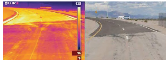
Figure 1: Thermal infrared (left) and visible (right) images of a road with light and dark segments. The infrared image shows that the light segment (bottom) is about 17°C (30°F) cooler than the dark segment (top). (Image courtesy of Larry Scofield, APCA)
