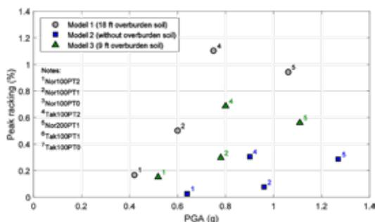
Image (e): Relationship of peak racking with peak ground acceleration in full-scale model dimensions (prototype)
