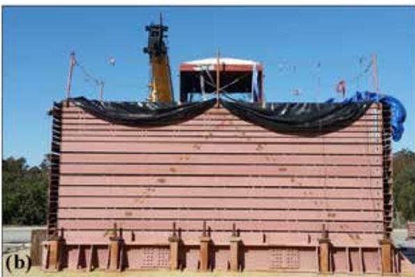
Image (b): Tunnel being lowered into large soil container
