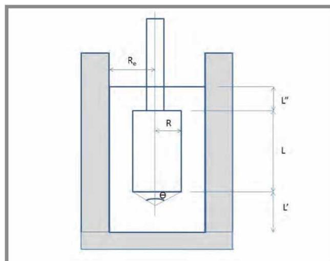
The proposed DSR concentric cylinder measuring system for evaluating asphalt binders has two cylinders: the inner cylinder is called the bob and the outer cylinder is called the cup.
