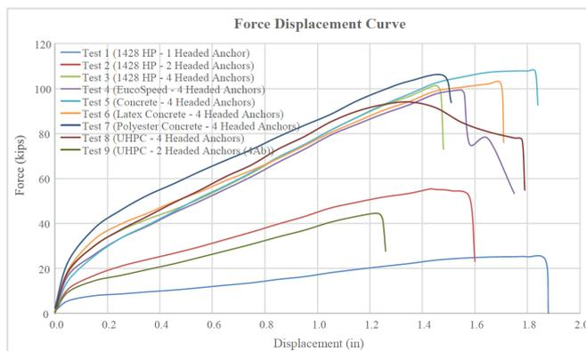
Image 5: Test results of shear force displacement response for all specimens
