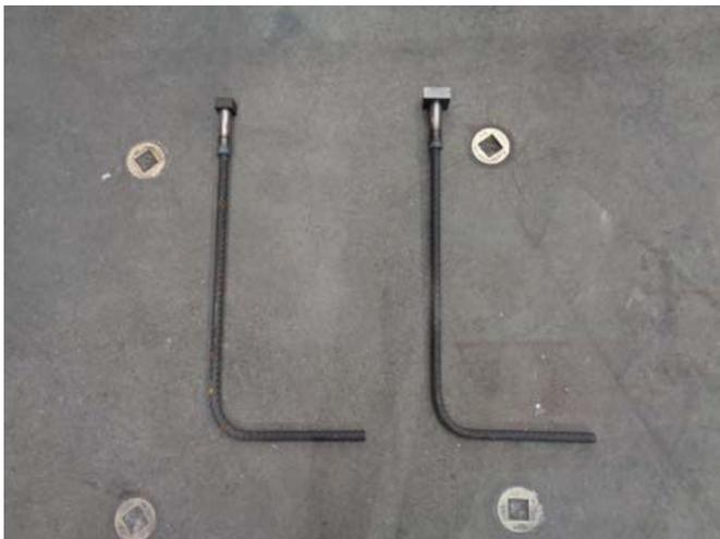
Image 3: Headed anchors used in the study (Left: Head Area = 4Ab; Right: Head Area = 9Ab)
