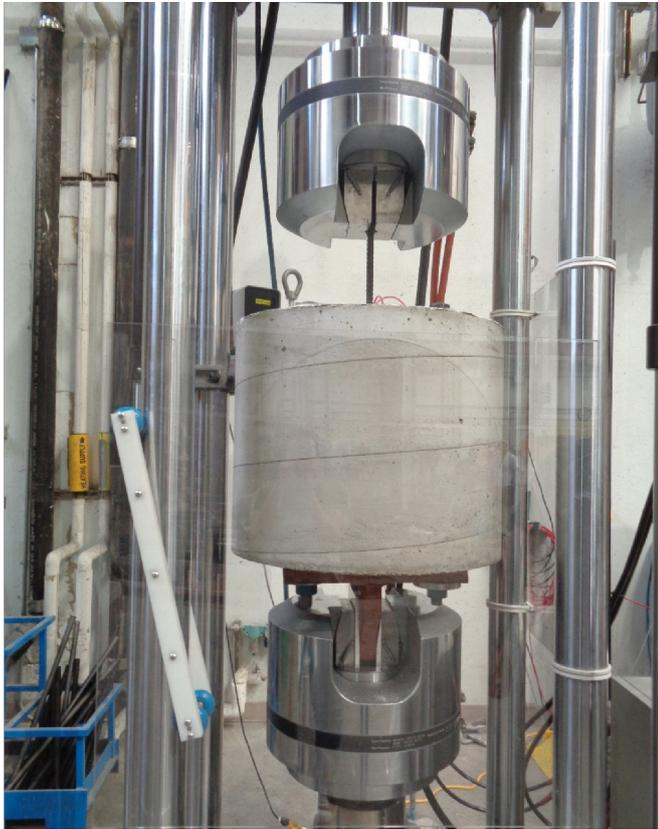
Image 6: Pullout test setup
