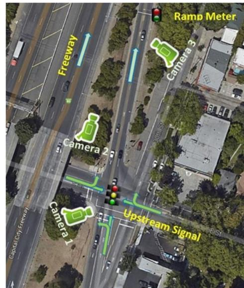
Image 6: Typical Camera Layout for Queue Storage Data Collection
