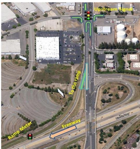
Image 5: Slip Ramp with Diverging Movement (Bradshaw Road to WB 50, Caltrans District 3)
