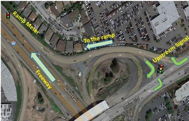
Image 4: Outer Diagonal Ramp with Two Feeding Movements (Marina Blvd to NB 880, Caltrans District 4)
