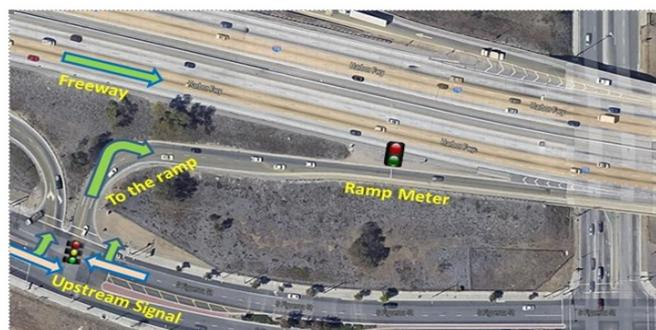
Image 3: Hook Ramp with Two Feeding Movements (Torrance Blvd to NB 110, Caltrans District 7)
