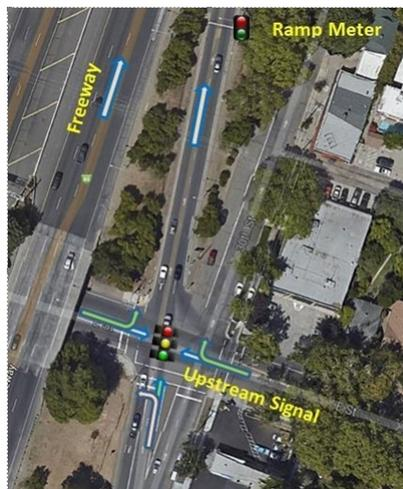
Image 1: Diamond Ramp with Three Feeding Movements (E St. to NB 99, Caltrans District 3)
