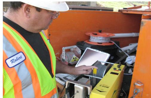
FIGURE 1: Mount Sopris Testing Equipment: Winch and Computer
