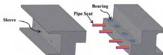
Figure 1: Pipe seat extenders in a typical in-span hinge
