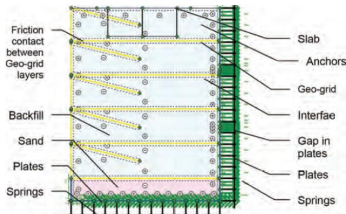
Figure 2: Geometry of the MSE model
