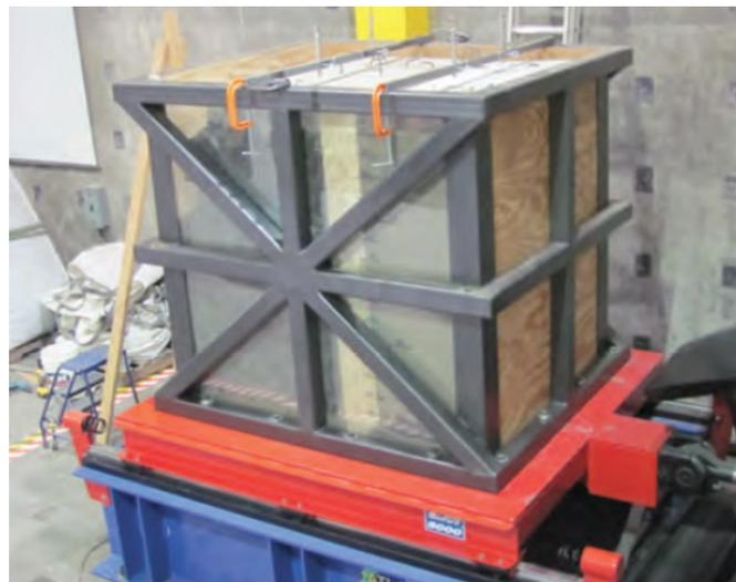
Figure 1: Shake table test of an MSE wall
