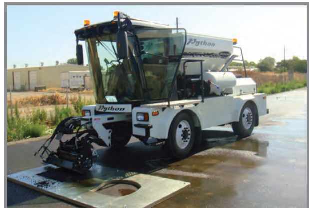
Python PHP 5000 Pothole Patcher during testing
