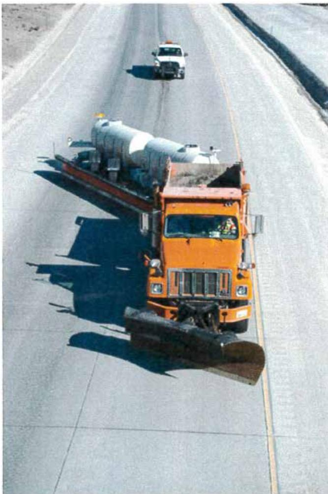
A TowPlow system in its deployed configuration
