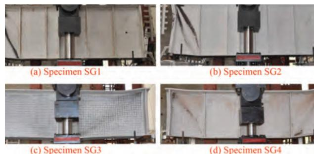
IMAGE 1: Failure modes of the steel girder specimens
