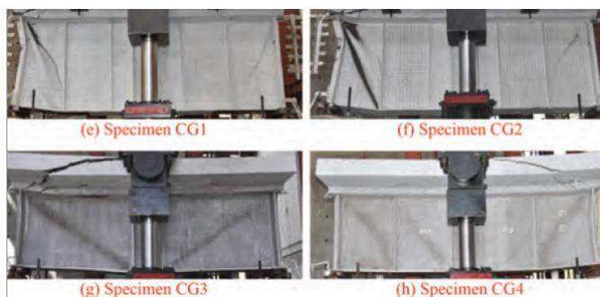
IMAGE 2: Failure modes of the composite girder specimens
