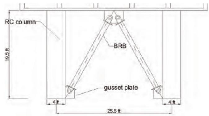
Figure 2: Transverse bridge bent with inverted-V BRBs
