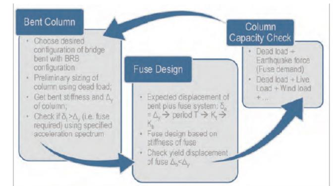
Figure 1: Design flowchart of bridge bent with buckling-restrained braces
