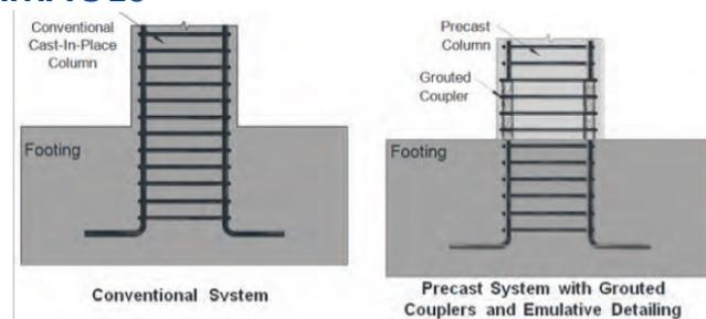
Figure 1: Comparison between conventional and precast systems with grouted coupler connections
