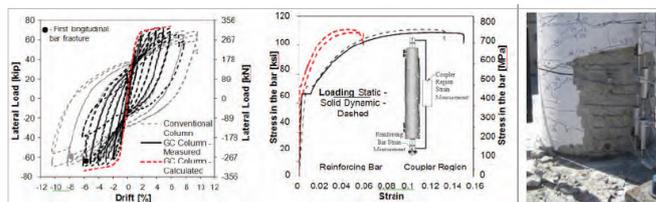
Figure 2: Behavior of grouted couplers and their connections (left to right): Force-displacement response of conventional and grouted coupler columns; tensile stress-strain response from individual couplers; damage of a grouted coupler column-footing connection at 6% drift
