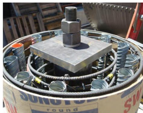
Figure 1: Pipe pin in pedestal
