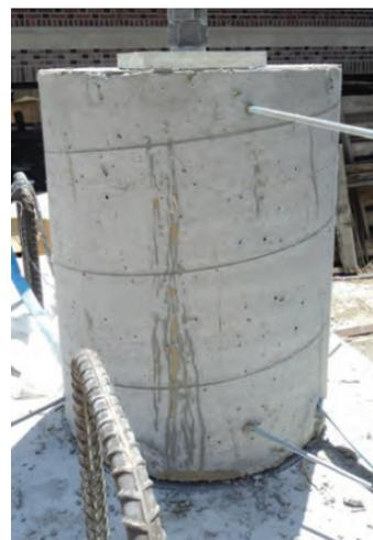
Figure 2: Pedestal with pipe pin connection at base
