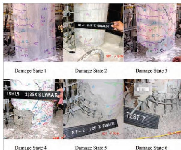
Figure 1: Possible apparent damage states of bridge columns
