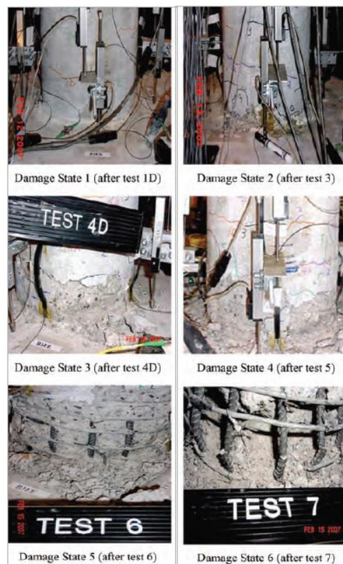
Figure 2: Damage states for bent 1 east column plastic hinge
