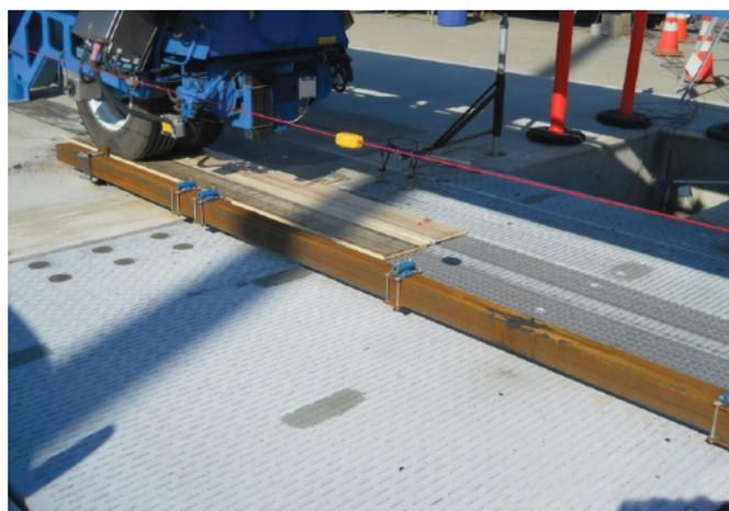
IMAGE 2: Close-up view of HVS testing on the deck joint
