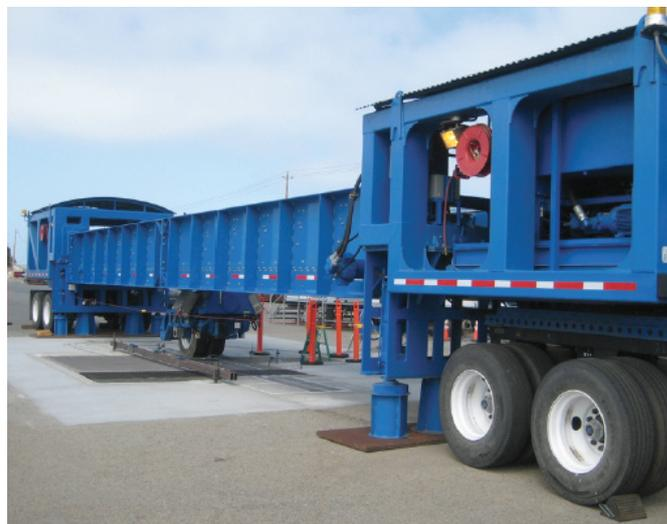
IMAGE 1: HVS testing on the deck joint
