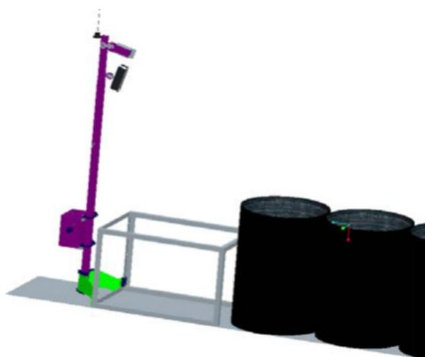
Image 2: Crash Attenuator Monitoring System
