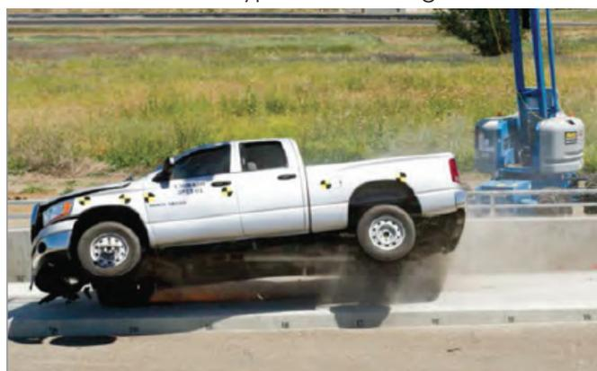
IMAGE 2: Pickup test impact
