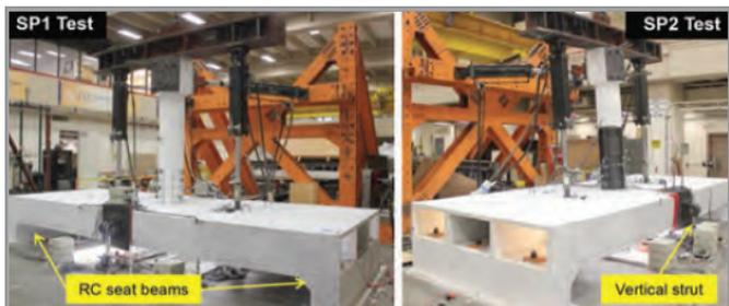
Figure 1: Cap beam, box-girder, column subassembly before bidirectional cyclic tests (left). Identical column repaired using a rapid carbon-fiber-reinforced polymer method during testing (right).
