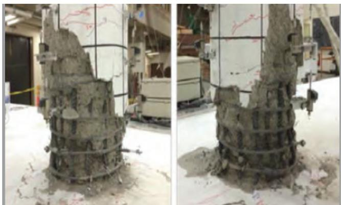
Figure 2: Column damage after cyclic tests
