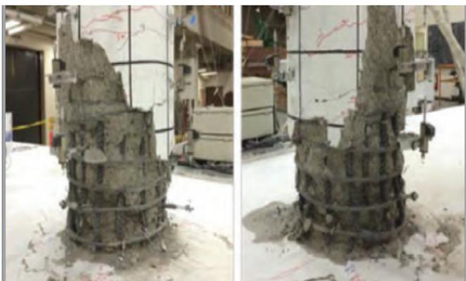
Figure 2: Column damage after cyclic tests
