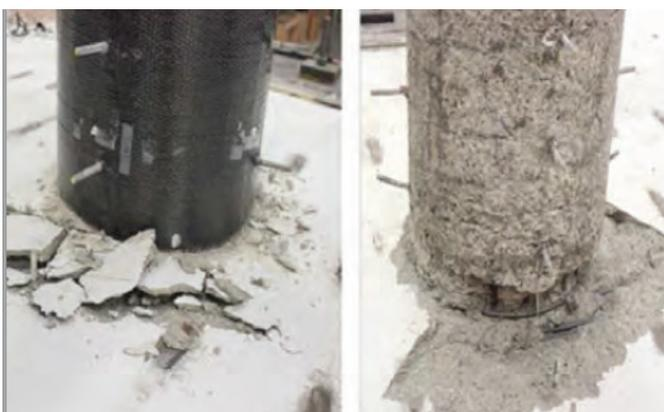
Figure 3: Cap beam concrete crushing and column flexural cracks (CFRP jacket removed) after hybrid simulation tests
