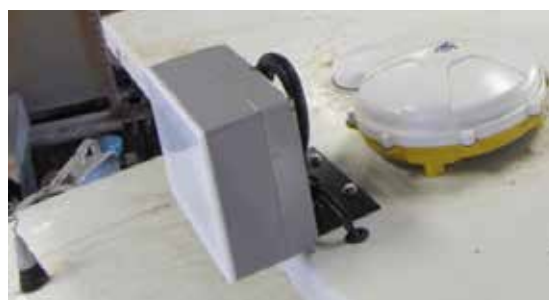
Figure 3: Radar, modem and GNSS antenna installed on top of a snowplow cab protector
