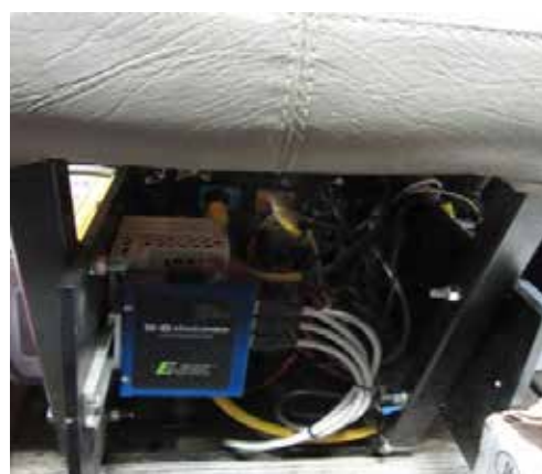
Figure 4: UM DAS computer installed underneath passenger seat
