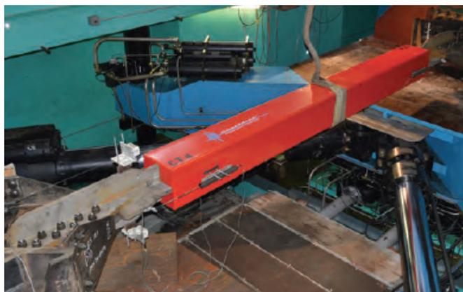
Figure 1: Left and right: Lab testing BRBs
