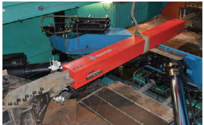
Figure 1: Left and right: Lab testing BRBs
