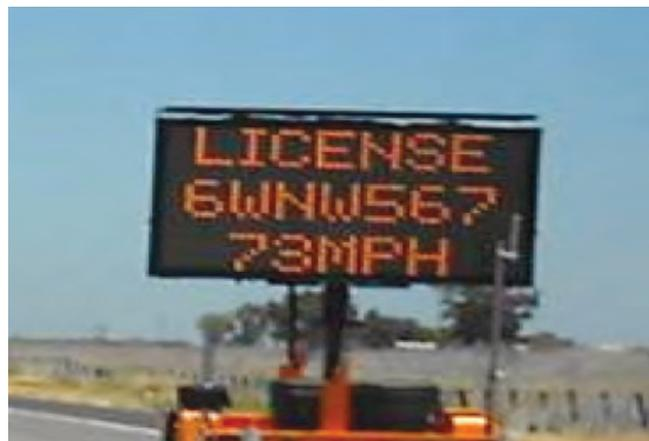
Image 1: The vehicle's license plate and speed are displayed on the changeable message sign.
