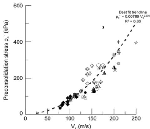
IMAGE 2: Relationship between preconsolidation stress and shear-wave velocity for clay.
