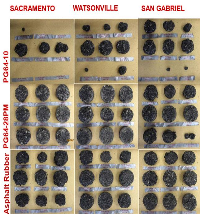
Image2: Photographic summary of Cantabro tests using Phase I SGC specimens
