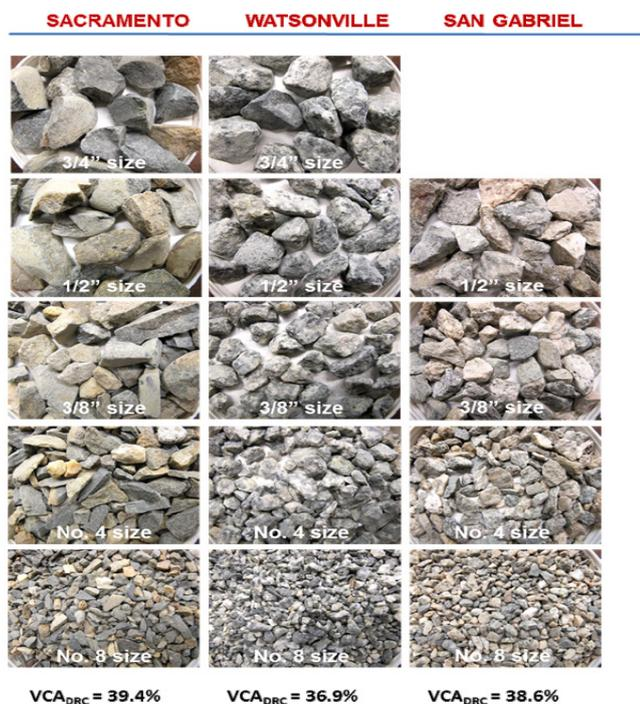
Image1: Three aggregates used in the tests per sieve size.
