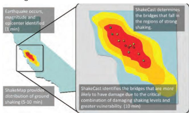
Figure 2: Sequence of ShakeCast analysis steps
