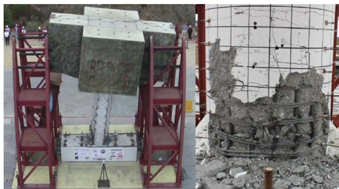
Figure 1: Close-up view of ductile fuse at column base after completion of all testing
