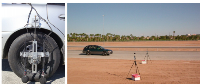
FIGURE 3 and 4: Locations of microphones for measuring tire-pavement noise (Left: measuring at the source using the OBSI method, Right: microphones for wayside measurements)
