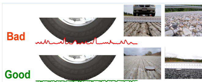
FIGURE 2: Conceptual schematic and photos of bad and good texture profiles as they relate to tire-pavement noise generation potential
