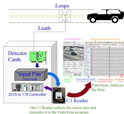
Figure 3: C1 Reader & VideoSync Vehicle Detector Analysis System
