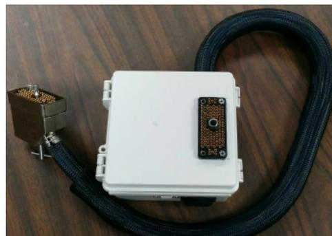
Figure 1: C1 Reader/Analyzer in Environmental Enclosure (closed)
