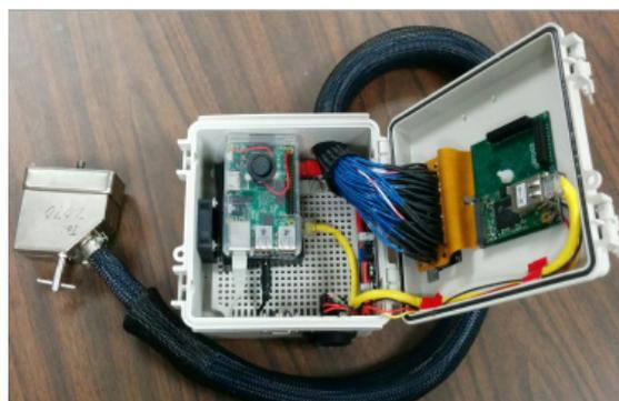
Figure 2: C1 Reader/Analyzer in Environmental Enclosure (open)
