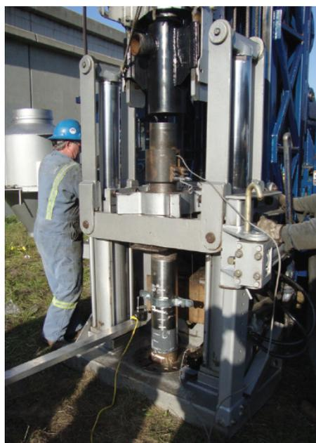
IMAGE 1: Drill ring with driving hammer in upward position
