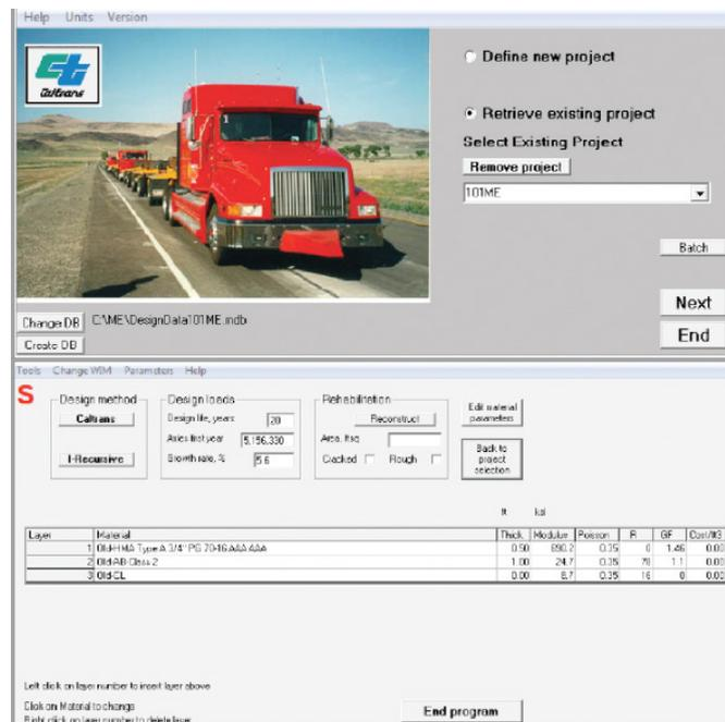
Figure 1: The CalME tool can analyze the use of different materials in the context of climate and load inputs and determine the cost.
