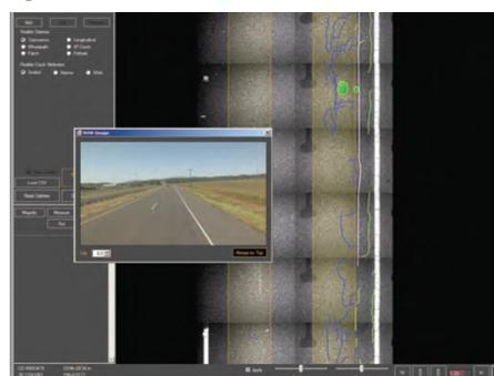
Figure 1: Crack map of a highway section
