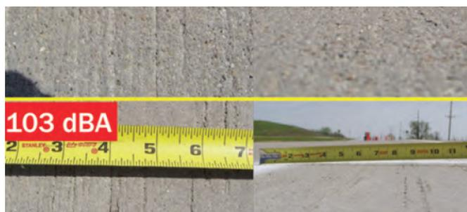
IMAGE 2: Variability of drag texture surface and its effect on overall OBSI level
