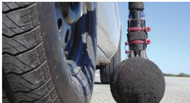
IMAGE 1: Measuring tire pavement noise
