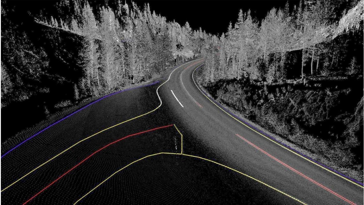
**Figure 2.3: Example 3D laser scan point cloud with extracted base map overlay**
