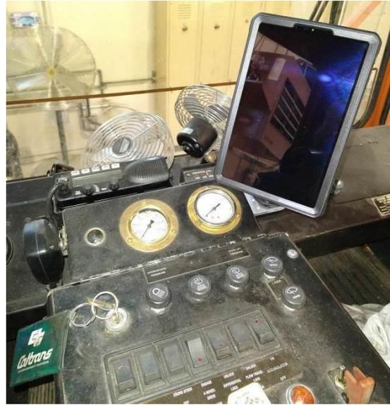
**Figure 3.9: Example MPRO system installation inside a snow blower cab**
