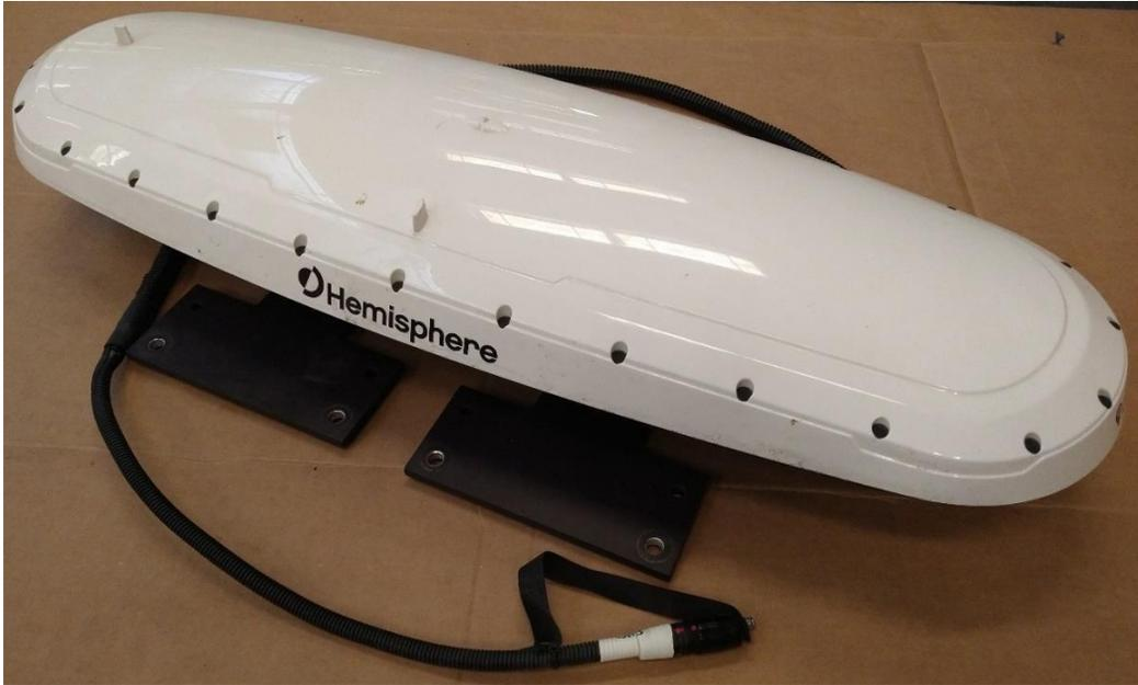
**Figure 3.2: Hemisphere Vector V500 GNSS Smart Antenna with M12 connector extension cable**
