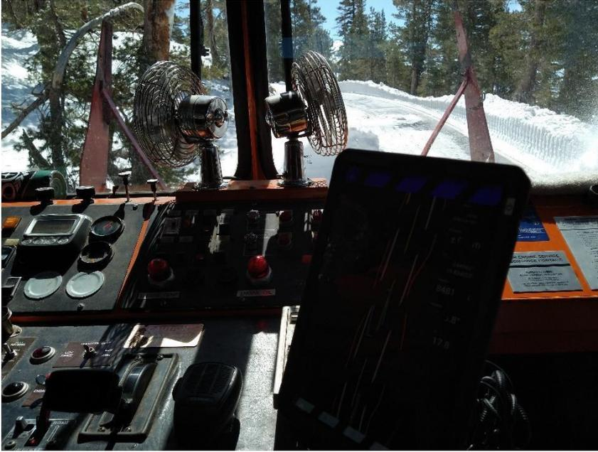
**Figure 5.1: MPRO system field testing at SR 4 on a snow blower. GNSS-challenged condition with dense tall trees on both side of the roadway. The display was in the middle of refreshing the display.**
