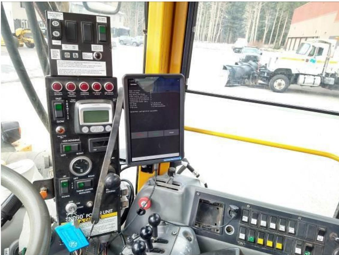
**Figure 3.10: Example MPRO system installation inside a front-end loader cab**
