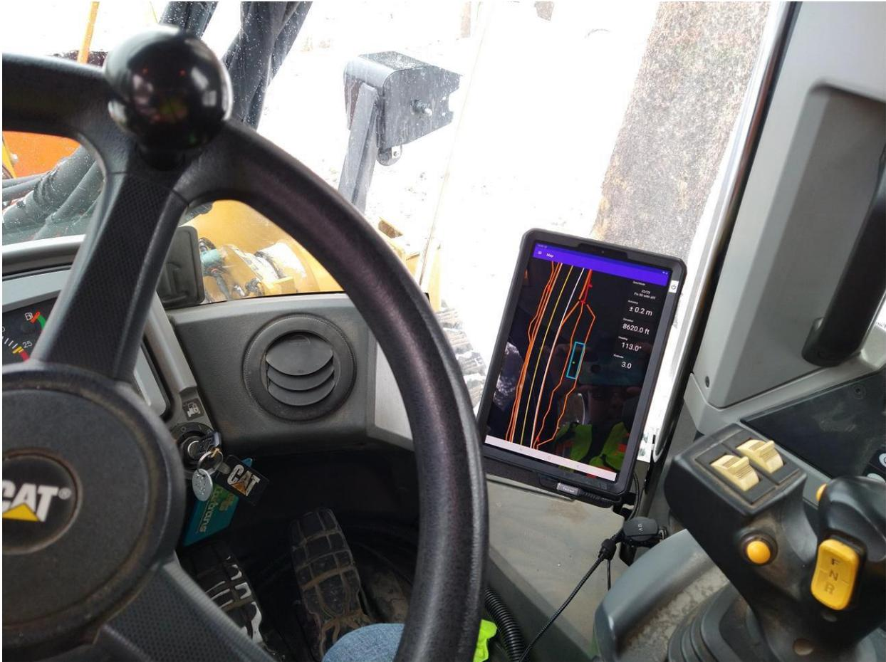
**Figure 3.13: MPRO system with active HMI inside the front-end loader**
