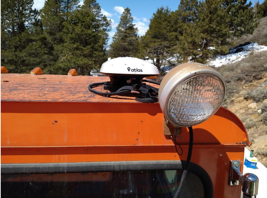
**Figure 3.5: Vector V500 GNSS Smart Antenna mount on a flat steel roof of a snow blower using magnetic mount**
