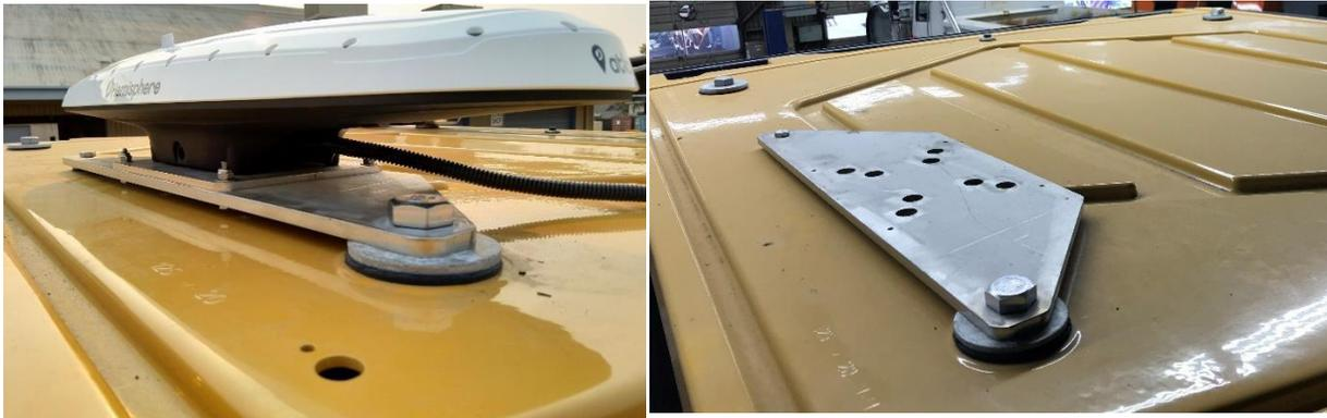
**Figure 3.3: Vector V500 GNSS Smart Antenna custom-mounted on a Caterpillar 950 front-end loader with fiber glass roof**
