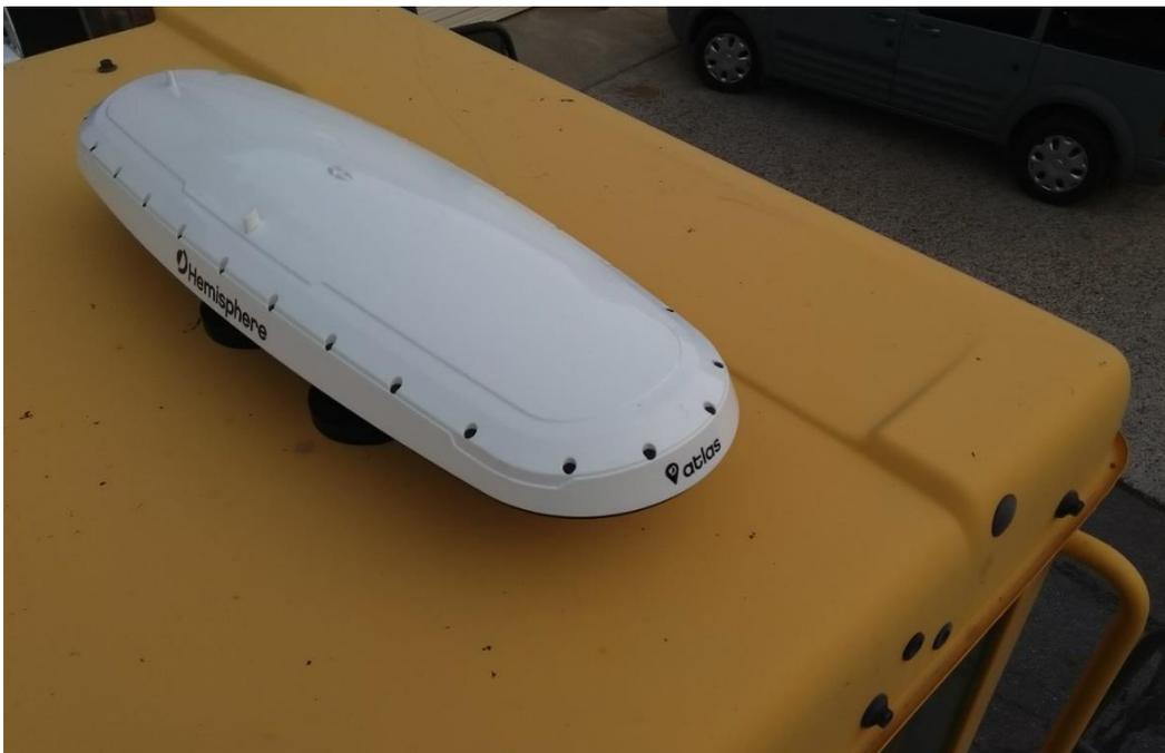
**Figure 3.4: Vector V500 GNSS Smart Antenna mounted on a flat steel roof of a front-end loader using magnetic mount**
