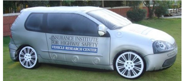
Image 2: Example of Obstacle for Testing (Inflatable Car with Foil Inserts)
