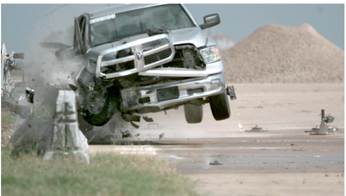
Image 4: Test 616811-01-4 PCC Bolted Median Configuration with 5 inch embedment 2023_09_29
