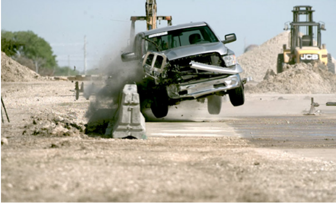
Image 2: Test 616811-01-2 PCC Bolted Roadside Configuration 2023_03_13
