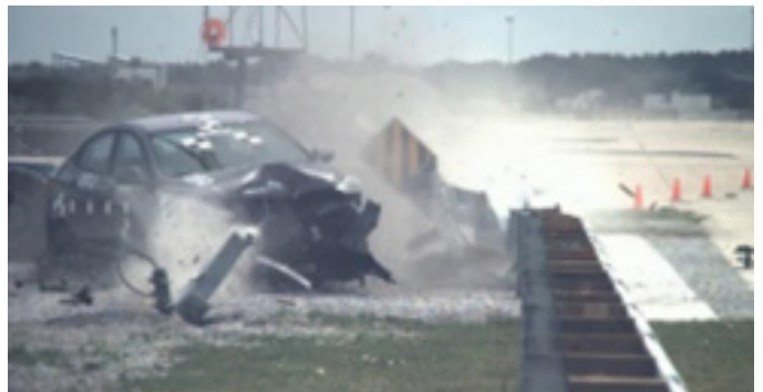
Image 5: Crash Test CET-2 (Test 3-32) During Impact
