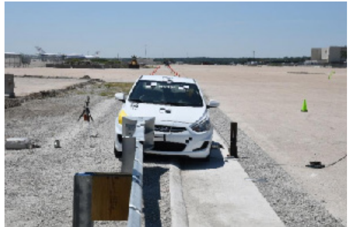
Image 2: Crash Test CET-1 (Test 3-30) Pre-Test
