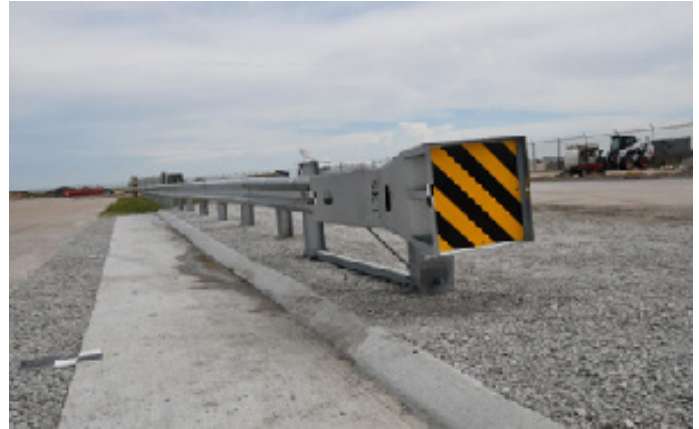
Image 1: Traffic Face of End Terminal with 4-inch Curb Prior to Test
