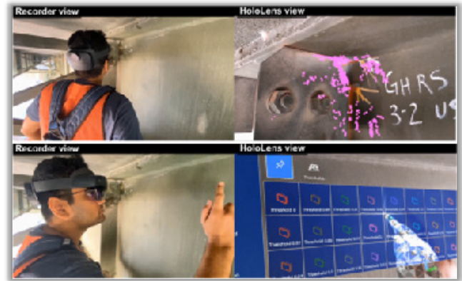
Image 2: Human-centered fatigue crack inspection tool developed under NCHRP IDEA 223
