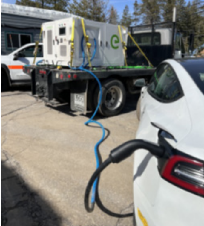
Image 4: Tesla Model 3 being charged by EVE-6060-NA charger.
