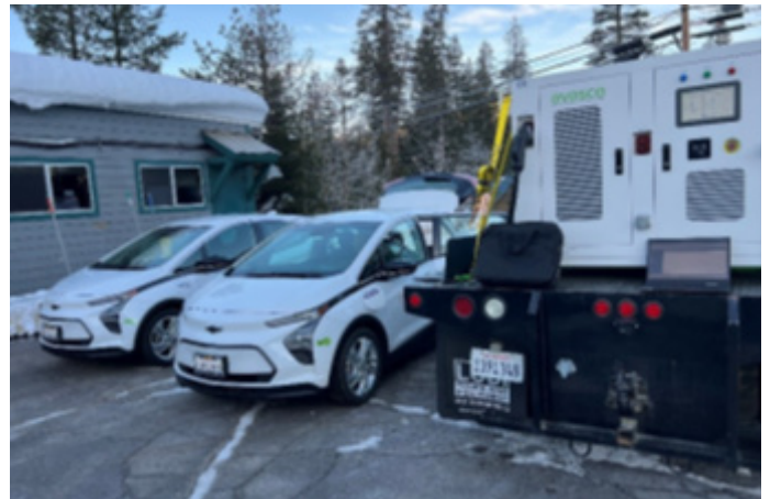
Image 3: Chevrolet Bolt being charged by EVES-6060-NA charger.
