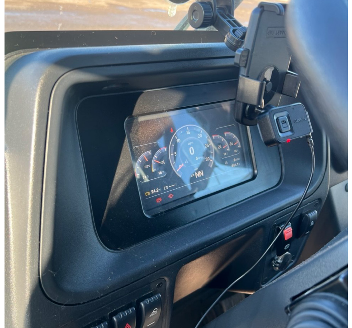
Image 3: Dash-cam view of the machine's digital dashboard used to monitor real-time battery state of charge (SOC), gear status, and temperature for operational timescale analysis.
