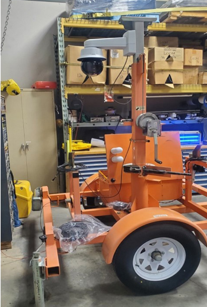
Image 1: Trailer-mounted camera and computing system prepared for field testing. (Source: UC Davis AHMCT)
