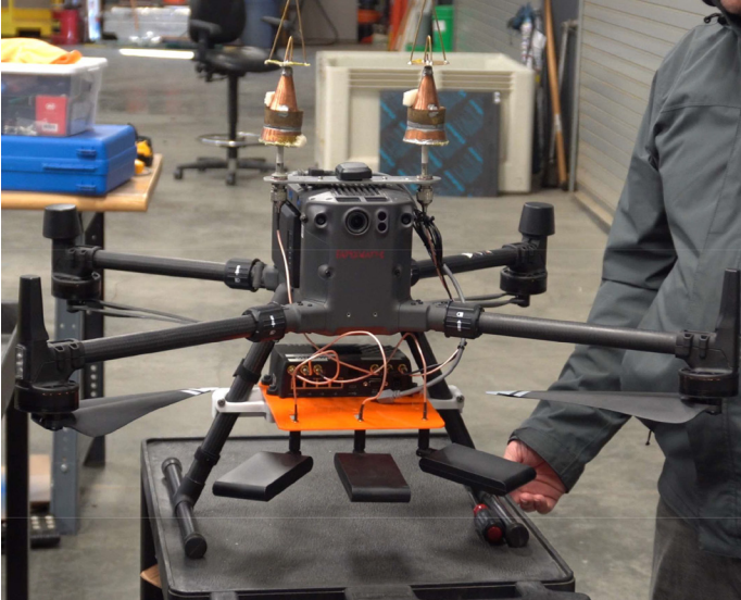
Image 2: DJI Matrice 300 RTK outfitted with cellular modem and WiFi repeater.
