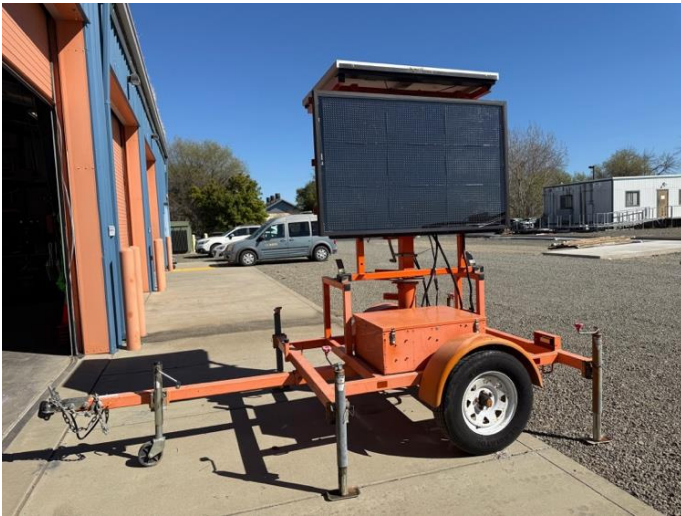
Image 1: Prototype trailer-mounted changeable message sign used for controlled testing of the Targeted Warning Messaging system. (Source: UC Davis AHMCT)
